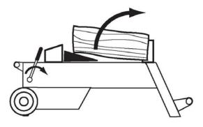
4. Lift the log off the wood splitter Wedge after loosening.
